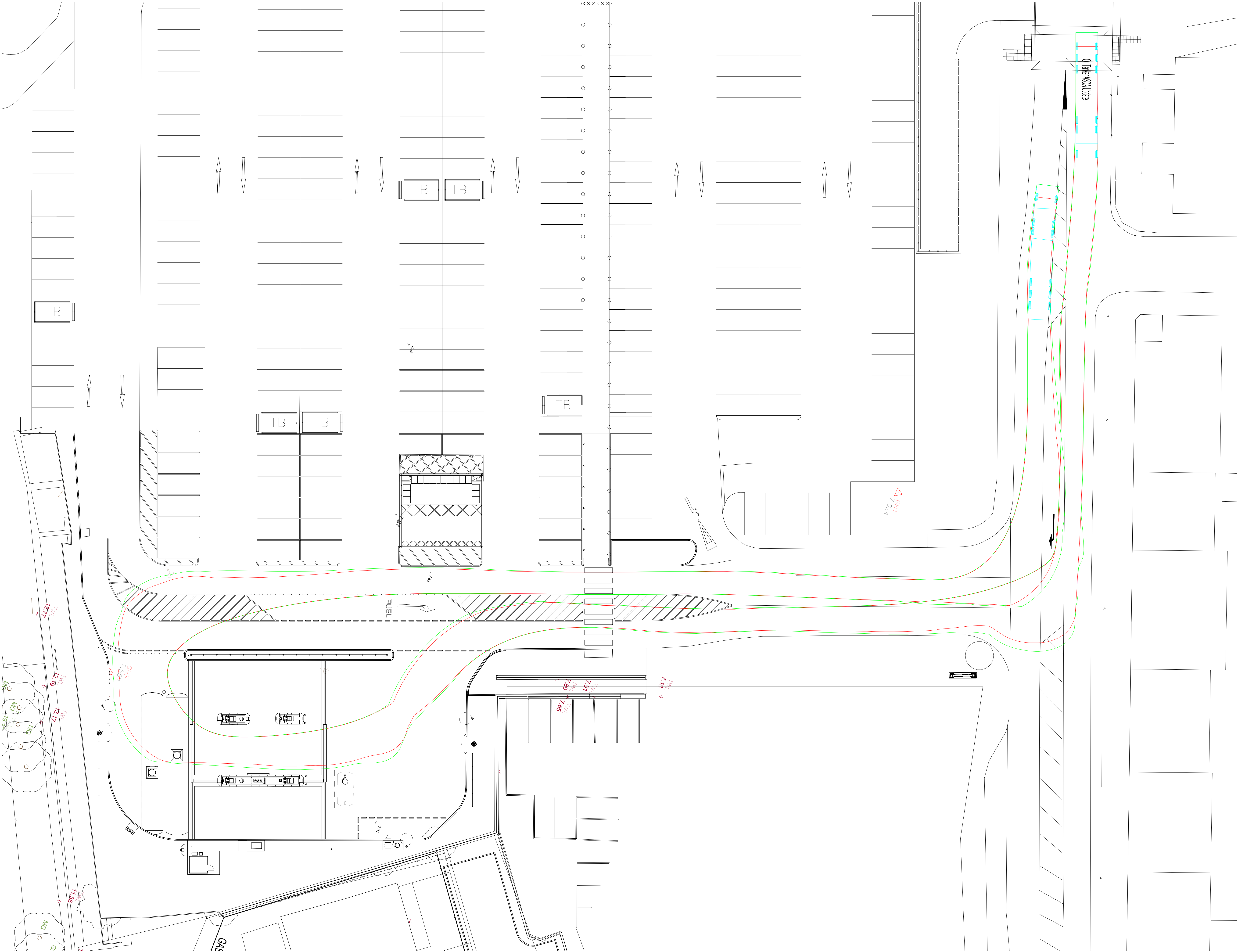
Tanker junction tracking 1 : 200
